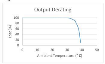
When internal temperature is higher than the limit, the thermal control system will gradually lower the intensity of the connected strips or dots to cool down the driver. Once the internal temperature is within the limit, the driver will resume its normal operation.
