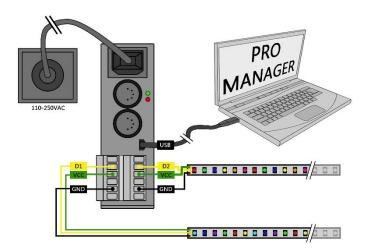
When connected by USB, it should be correctly identified as ENTTEC Pixie Driver by your computer. Please install and run PRO-Manager with the Pixie driver connected.
