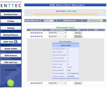
RDM tools page, with DMX ports set as output, can be used to discover RDM device, and allow user to access and control below 10 PIDs without relying on external RDM controller. Each RDM device, has its' own set of functions and buttons, so multiple devices can be handled easily. Clicking on the device ID, opens a new page to handle this device separately.
