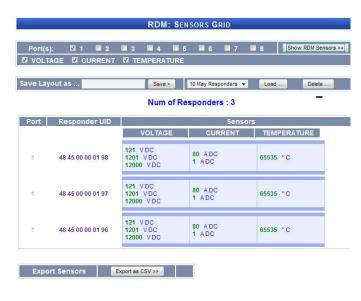
RDM Sensors page, allows discovering all RDM devices and monitoring all sensors supported by RDM tool. Examples include: Temperature, Current and, Voltage sensors.
