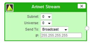
Art-Net Stream: "Send IP address": is the destination address used when the stream is sending data only (Unicast).
