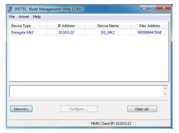
NMU (Node Management Utility) is a free Windows and OSX application that is used to manage compatible ENTTEC DMX over Ethernet nodes.
