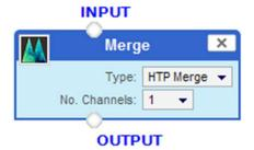
Merge: HTP or LTP merge operator, drag as many lines to the input node as you wish to merge
