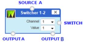
Switcher 1-2: Controllable Switch operator, when the trigger channel (Switch) is greater than the set value, OUTPUT B is output, in other cases OUTPUT A is output. Must have all input sources and output sources connected
