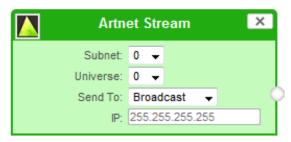
Art-Net Stream: "Send IP address": is the destination address used when the stream is sending data only (Unicast).
