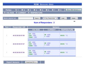
RDM Sensors page, allows discovering all RDM devices and monitoring all sensors supported by the RDM devices found. Examples include: Temperature, Current and, Voltage sensors. The displayed sensors values are refreshed, automatically every few seconds.
