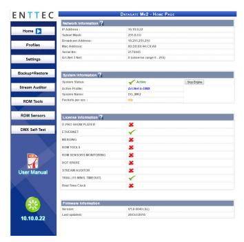
The Datagate Mk2 is configured, controlled and programmed through a web browser interface running on a computer system located on the same Local Area Network. Any modern web browser, such as Chrome, Firefox, Internet Explorer, Safari or Opera, running under any operating system, including Windows XP or Vista, Mac OS X or Linux can be used.
