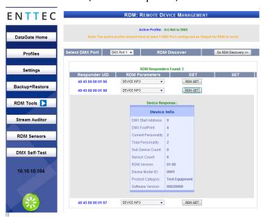
RDM Tools page, allows access to RDM functions on the Datagate Mk2. All DMX ports set as output, can be used to discover RDM devices, and change the common RDM options such as: DMX address, Personality and Identify.
