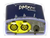
For your convenience the interface has two DMX output sockets, a 3-pin XLR and a 5-pin XLR. This allows you to connect your lighting rig using either 5-pin or 3-pin XLR cables. (Although the official DMX standard specifies 5-pin connections, many lighting manufacturers routinely use 3-pin connections on their most popular lighting fixtures).
