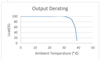
When internal temperature is higher than the limit, the thermal control system will gradually lower the intensity of the connected strips or dots to cool down the driver. Once the internal temperature is within the limit, the driver will resume its normal operation.
