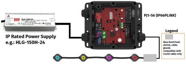
9PDOT1 IP67 rated RGB 24V pixel dots
