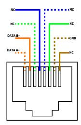
Plink Punch down pinout with T568B colour code
