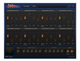
Masked channels appear greyed-out on the DMXIS display. This screenshot shows a preset where only the **Shutter** channels on the RGB fixtures are enabled.
