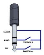
Only use passive pedals that simply short-out the tip & sleeve (Switch A) or ring & sleeve (Switch B) of the ¼" jack. Do NOT use any proprietary type pedals which do not a standard mono/stereo ¼" jack connections, or which transmit any additional power or control signals along the cable.
