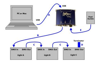
A: Connect the DMXIS hardware interface box to your computer with a USB cable.
