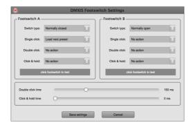
This window is accessed from the standalone DMXIS program (*Footswitch - Footswitch Settings* menu on OS *X, File - Footswitch Settings* menu on Windows). The settings applied here will also be used for the DMXIS plug-in.
