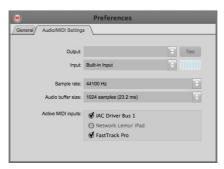
Here you specify the audio driver and audio latency used by the DMXIS standalone program. For accurate DMXIS operation, you should ideally specify an audio buffer size of approximately 25ms / 1024 samples or lower.
